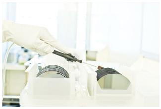
Fig. 3 - Lifting the Wafers with Vacuum Tweezers
