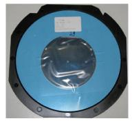
Fig. 2 - Sawn Dice on Disco Frame
