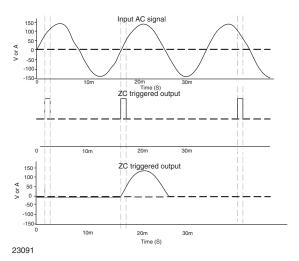
Fig. 29 - Zero-Crossing Modulation Control
