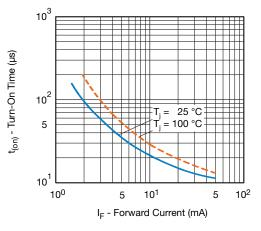
Fig. 1 - Turn-On Time vs. Forward Current
