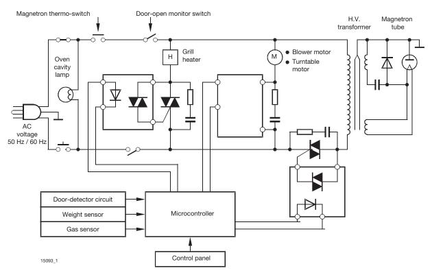
Fig. 34 - Microwave Oven With Grill Example
