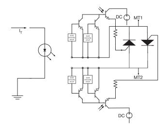
Fig. 9 - Phototriac Functional Diagram
