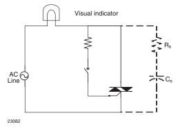
Fig. 17 - Simple Static Switch Application
