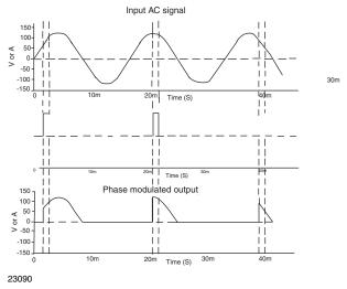
Fig. 28 - Phase Modulation Control
