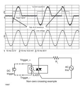
Fig. 10 - NZC TRIAC Waveforms
