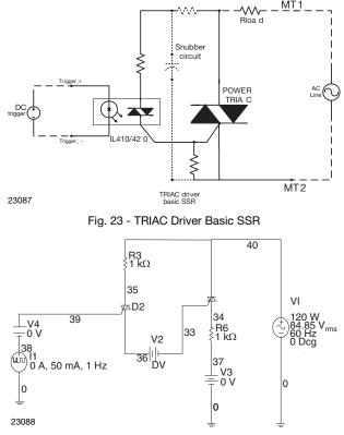
Fig. 24 - In Depth TRIAC Driver Model
