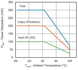
Fig. 30 - Allowable Dissipated Power
