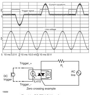
Fig. 11 - ZC TRIAC Waveforms
