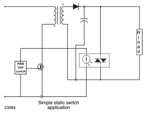
Fig. 19 - Simple Static Switch Application
