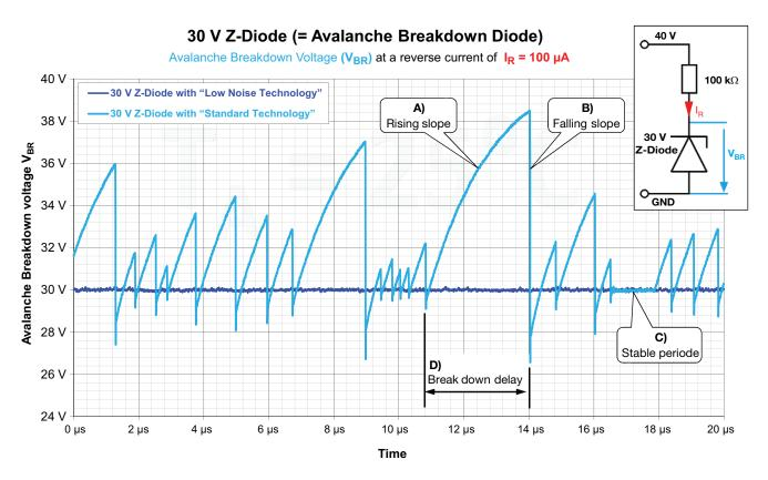
Fig. 1 - Breakdown voltage of one Z-Diode with and one without "Low Noise Technology"
