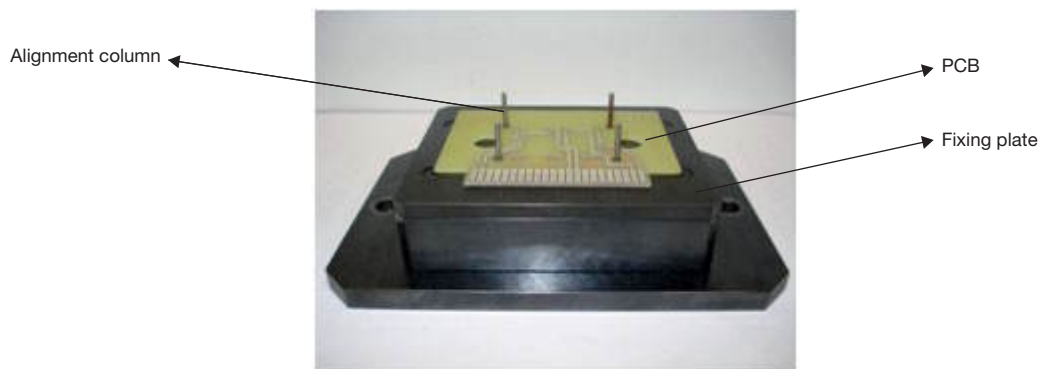
Fig. 6 - Step 1: Put the PCB on the assistant tool
