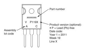
Example: This is a xxxxxxx with assembly lot code AC, assembled on WW 19, 2011 in the assembly line "X"
