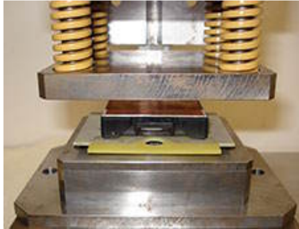
Fig. 11 - Step 4: stop the machine and press-in is finished
